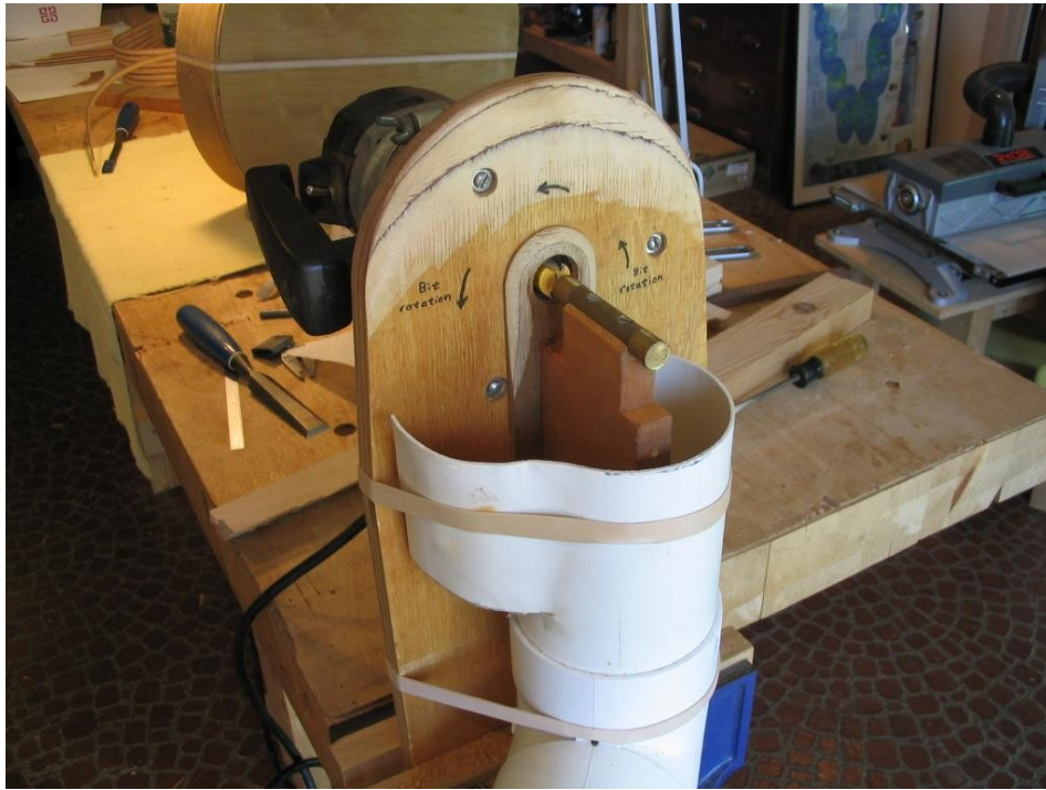
Figure 4: Shop-made Larrivee-style binding jig
