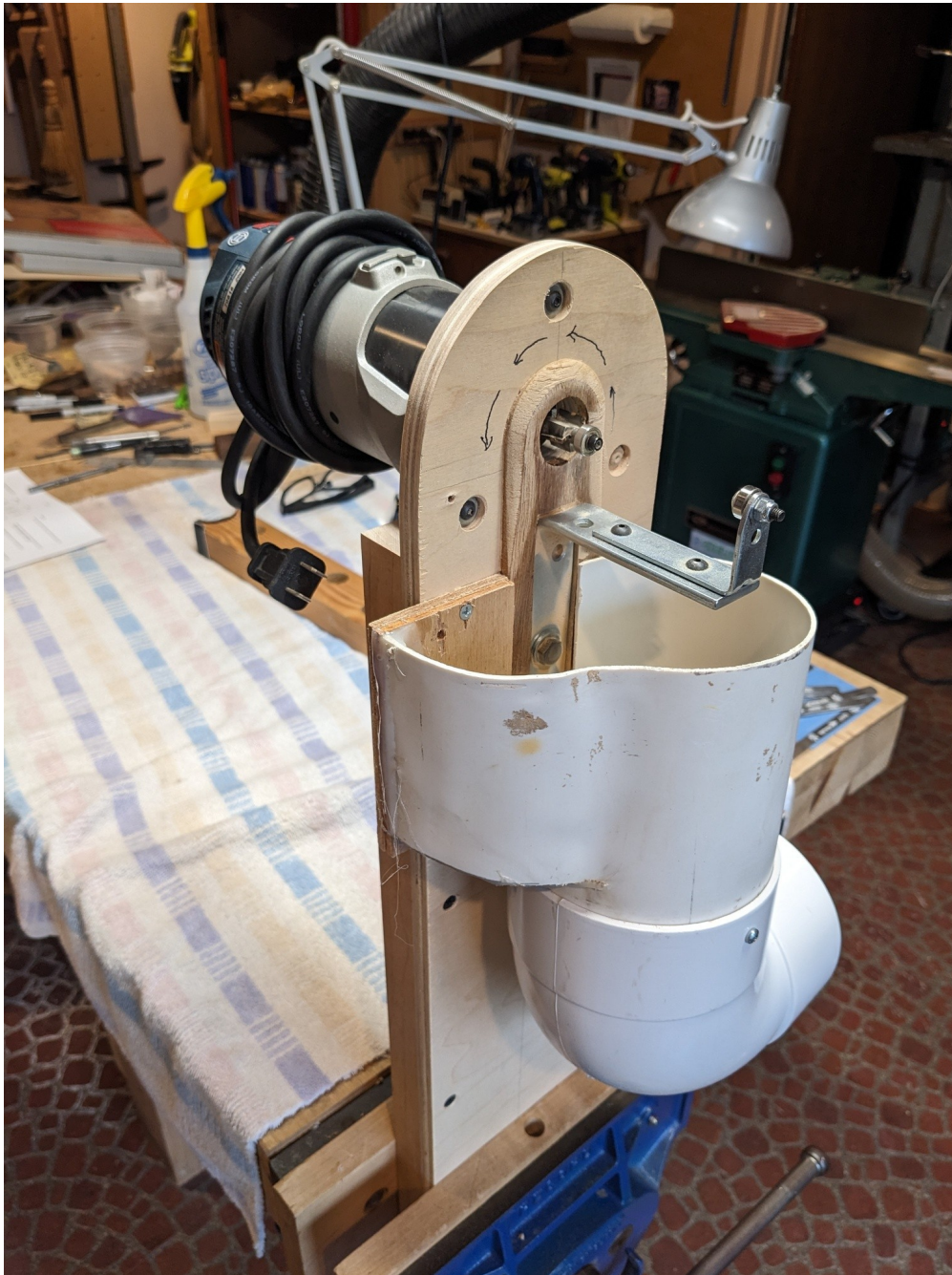
Figure 7: Modified Larrivee-style jig with bearings replacing guide rod
