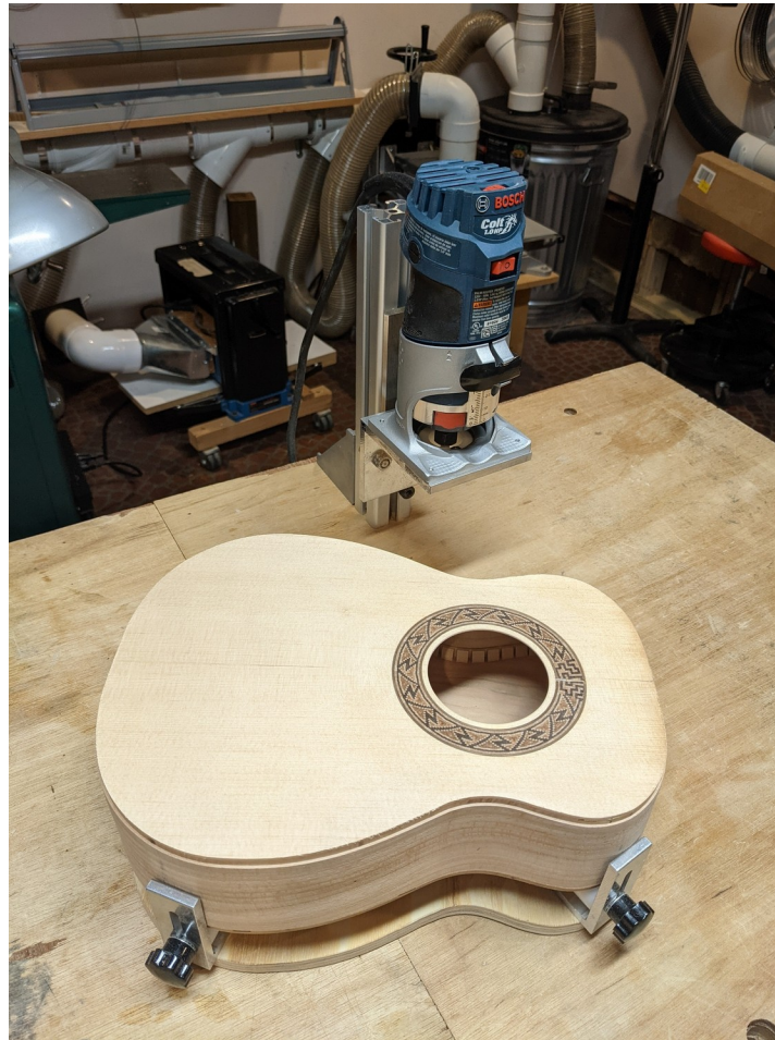
Figure 5: Elmer Guitar tower-and-sled binding jig
