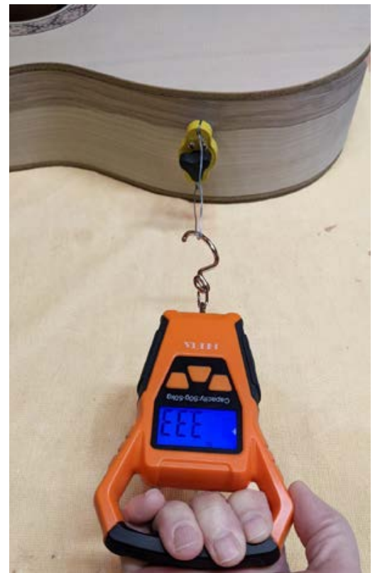
Photo 3. Measuring release force for a guitar side. The steel rod is inside the body.
