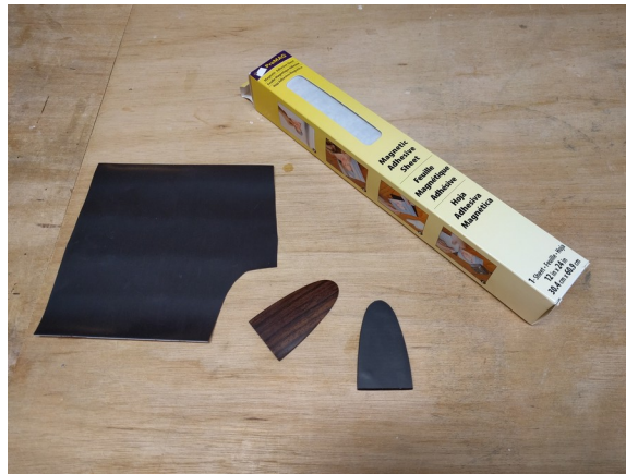
Cover plate with self-adhesive magnetic material on the back
